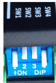
Figure 8 DIP switch for braking voltage configuration
