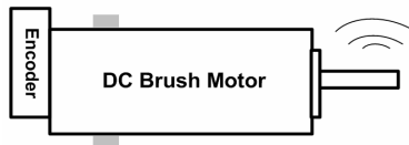
Figure 6-27: Observe the motor noise/vibration when increasing loop gain
