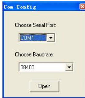
Figure 6-11: RS232 communication configuration window
